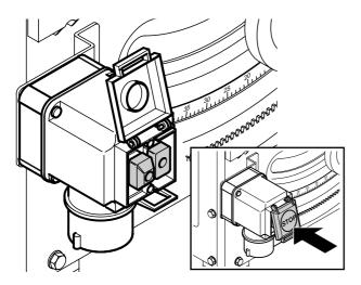
An undervoltage relay trips in the event of a voltage failure, to prevent a restarting of the saw when the power is restored. To start the saw again after a power failure press the green button.
